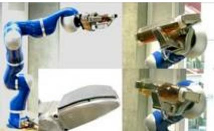
UEDIN developed a framework for discrimination of dynamic object properties based purely on the learned sensorimotor contingency representation of actions and tactile sensor activations (Saal, Ting, & Vijayakumar, 2010a). This was used to not only discriminate between liquids of different viscosity (e.g., water, motor oil and glycerin of equal weight in a bottle) but also used to implement an info-max
