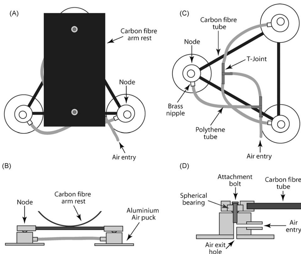
**Fig. 5.** The air sled. (A) and (B) show the top and side views of the air sled, respectively. (C) shows plan view with arm rest removed for clarity. Air flow resistance was balanced by the use of two T-joints. (D) shows a cross section through an air puck including its attachment to a support node. Air flows in via a brass nipple and out through a hole in the base. A spherical bearing is used to connect the puck to its support node, allowing it to align with the surface of the air table.
