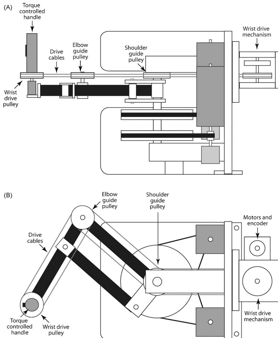
**Fig. 3.** Anatomy of the WristBOT, showing additional cable drive mechanism. (A) Side view showing the cable routed from the handle, via the guide pulleys, to the drive mechanism mounted on the base plate. (B) Top view.
