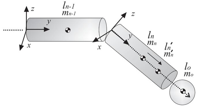
Fig. 4. In our experiments, both the center of mass of the last link  $l_n$  and the load  $l_o$  are constrained to lie on the  $y$  axis of the last link's reference frame, so that the center of mass of their union  $\hat{l}_n$  also lies on the  $y$  axis.
