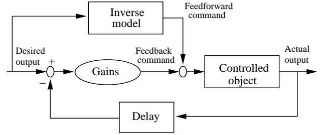
Fig. 1. The composite controller
